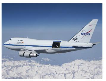
Fig. 1 The SOFIA B747SP aircraft with open door flying over the Sierra Nevada in California (photo NASA).
